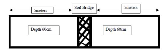
The cut off drain design can be improved by planting grass on the embankments to filter the silt from the running water. This maintains the shape and depth of the cutoff drain. For more effectiveness, there is need to provide a contour drain about five meters down slope from the cutoff drain.
