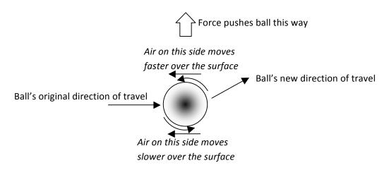
What does this have to do with aeroplanes? The LIFT force that keeps a plane aloft is very similar to the force that causes a football to bend. When the air is made to turn direction around some object like a football, it pushes sideways on the object.
