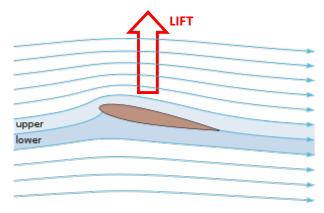
You can see that the air bends up over the top of the wing, but it also bends underneath too. So the air is rotating or curving a little bit.
